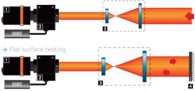
→ Optics quality control in double-pass: lens, objective, telescope in any size and magnification
