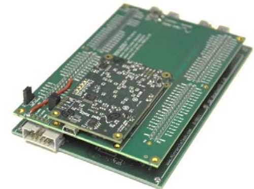
FPGA-based USB MEMS and Laser Controller
