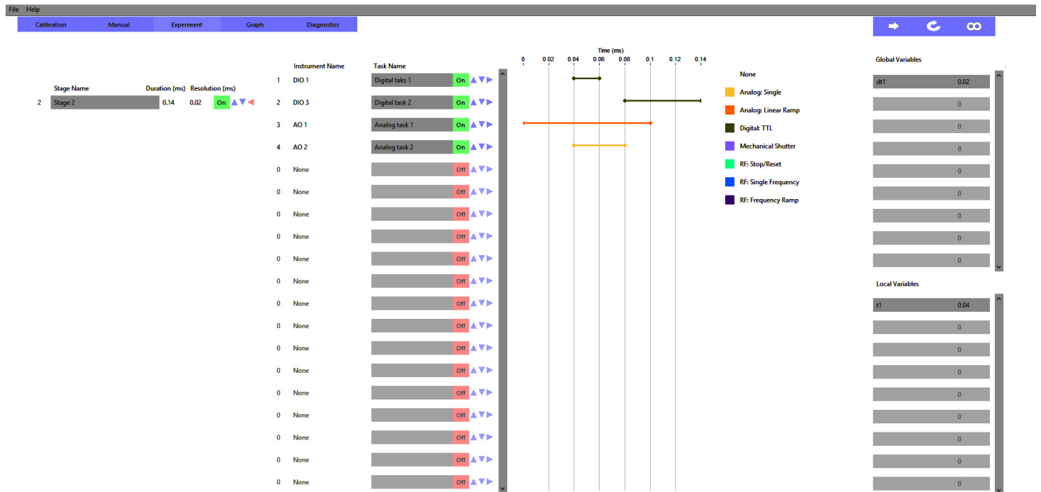
Screenshot of the QuCAL control software, showing the tasks, their respective channels, a timing Gantt chart and the Global and Local variables used to define the experiment.
